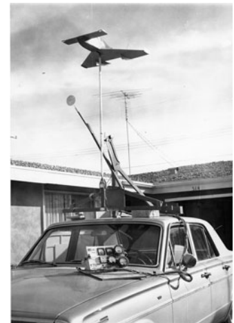
VariViggen Car Tunnel Model, showing the instruments to measure the effect of wind.
