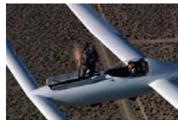
The Solitaire's retractable engine.
