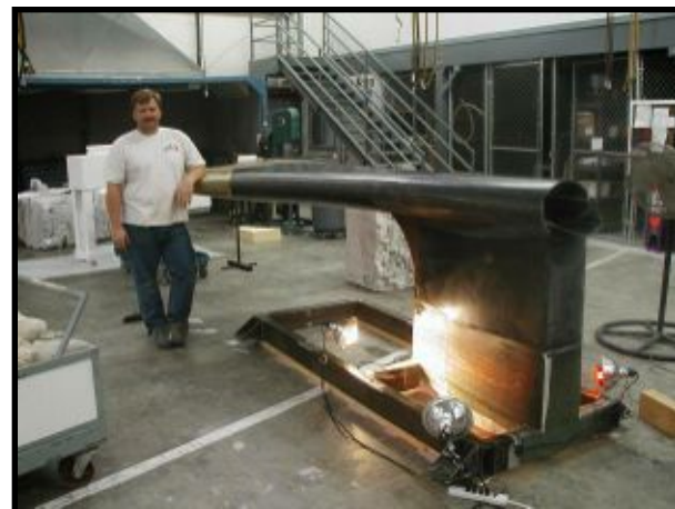
Static load proof, feather structure.
