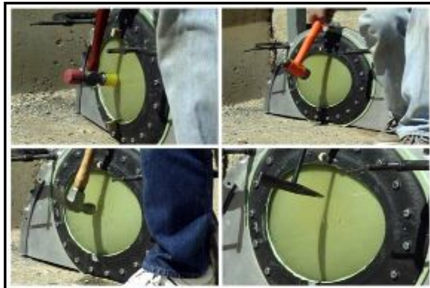
Window Damage Tolerance at 2x operating pressure (proof test at 3.5x)
